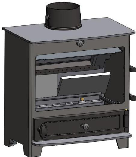
Pull the top edge of the Rear Brick forward and lift out of the Stove.
