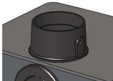
Place the Flue Gasket on the top, or rear outlet as required. Place the Flue Collar on top of the Gasket. Secure to the four locating tabs, inside the flue outlet, using the M6 nuts & bolts supplied. Fit the 2 - M8 carriage bolts, washers & nuts into the Damper Holes, located on each side of the Flue Collar.
