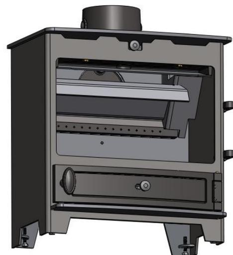
Slide the Baffle towards the front of the stove until it clears the Baffle Supports. Lower the Baffle into the Fire Box and remove.
