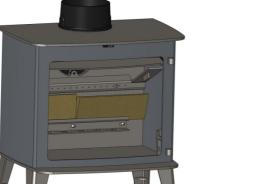
Pull the top edge of the Rear Brick forward and lift the brick out of the Stove.
