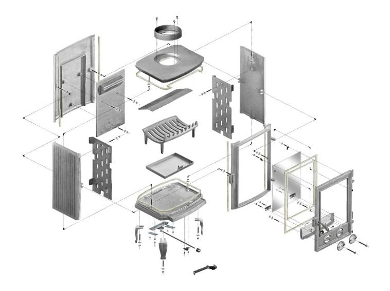
NB: The main part of the stove comes pre-assembled. The only parts which do not come assembled are the legs, the hood handle and the accessories.
