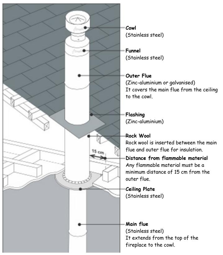
3. The flue pipe should be as straight and vertical as possible. If required, you can use up to two 135° bends. The vertical path should be twice as long as the horizontal. All bends should be after the first length of flue and before the outer flue commences. To ensure optimal performance, the length of the main flue should be between 4 meters and 11 meters in length. Do not place any turnbuckles or regulators on the main flue, since they can alter the fireplace's performance.
