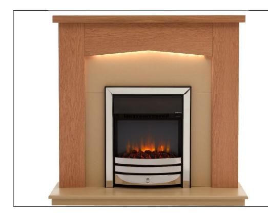
**Step 7.** Install the fire from front of the mantel. Note the fire must be fixed in position. Two screws should be positioned as detailed in the fire instructions to locate the fire on its key hole slots on the rear of the front frame.
