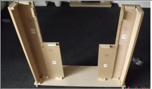
**Step 2.** Fix the second left and right panel (E&F). using 3 screws for each panel.
