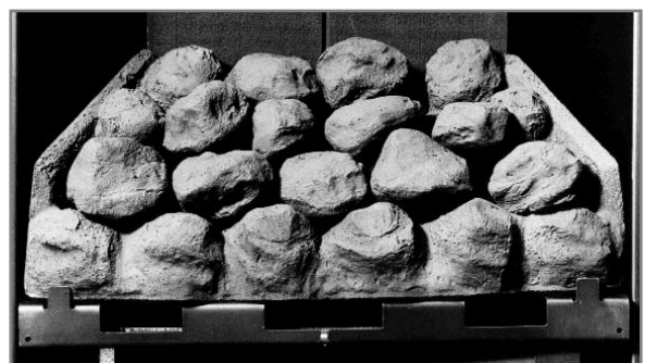
Place the middle row of four coals onto the supports in the matrix, over the top of the holes. Ensure the coals are not turned sideways, such that they actually enter the holes.
