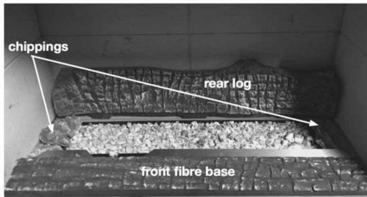
Rear log sits at back in channel as shown ensure air inlet is not blocked
