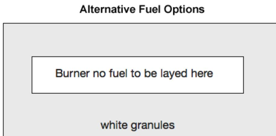
Alternative fuel options are available for these models and can be installed around the gas burner where the white granules are lay ,under no circumstances must the fuel be put across or in the burner .
