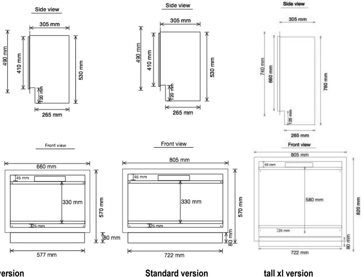
**ALL MODELS HAVE A 25mm AIR SUPPLY AT THE FRONT BOTTOM UNDER NO CIRCUMSTANCES SHOULD THIS BE BLOCKED OFF AT ANY TIME**
