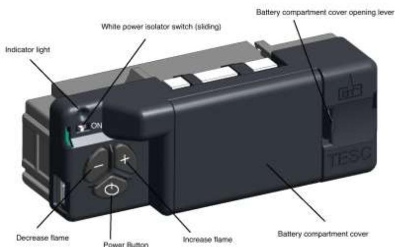
After fitting the batteries and replacing the cover the fire can now operate. Slide the slide switch to the right to the On position (I symbol).
