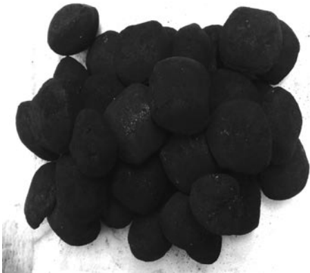
Recommended maximum smokeless fuel load: approx 1.75kg of approved smokeless nuggets
