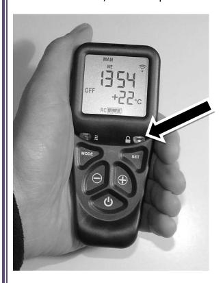
**3) Setting the time** the display will be as shown, as the time is not set yet and will progress automatically to the next screen shown below.
