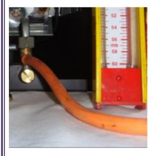
Check that the standing inlet gas pressure is at 20 mbar
