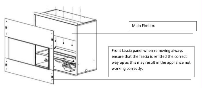
You will need to remove the plaster from the wall around the fire enough to be able to fix a sheet of master board or non- combustible board over the fire box when in place to be able to be plastered to a finish ready to be decorated.
