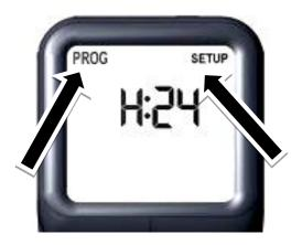
Press and Release the "Set" button several times until you see CAO displayed. Then press and release "+" button once to change display to CA1 Press and Release the "Set" button once more to display TESC, handset is now ready to pair.
