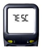
**1a)** if display is not as above the handset may well need to be reset before pairing. Press and Hold "Set" Button, to enter Programing menu When Set Up is flashing, press and release set to enter Setup Mode.
