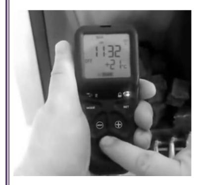
Press and hold in the power symbol button and release immediately when the word pilot appears at the bottom left of the display (after about 1-2 seconds). The fire will light.
