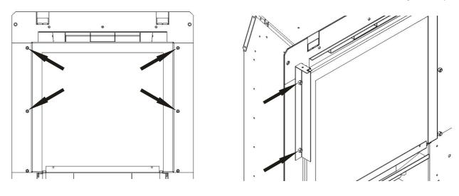
Place glass fascia on the fire as shown below, be sure it is attached on bottom hanger and supported on side brackets as shown over page
