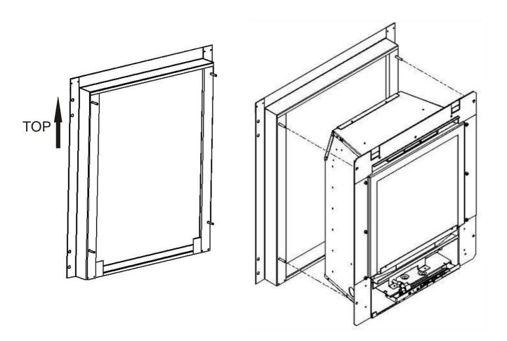
Then put fire into opening, mark, drill holes and fix to the wall with screws provided.
