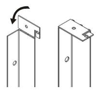
Remove the 4 nuts show below and reuse them fix side brackets to the firebox. **Note:** start fixing with top nut first!
