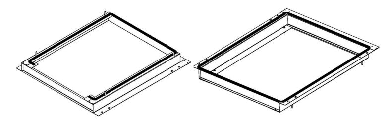
Assemble together firebox and spacer as shown below, secure bolts with M5 nuts provided.
