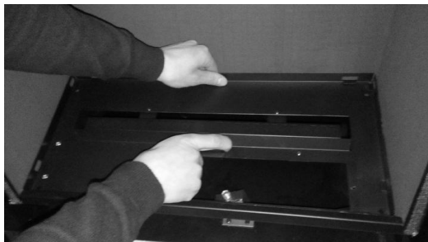
Fig 5. Carefully remove the burner tray by lifting the back of tray first
