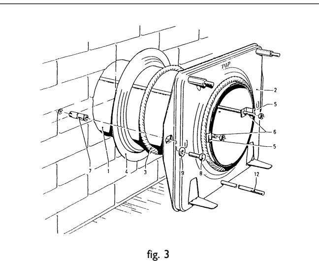
sheet up to the wall. Press the inlet pipe back in such a way that the end of the pipe is level with the turned-back edge of the mounting sheet.
