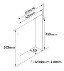
5.5 Carefully mark out the fixing screw positions as above, fit two pan head screws leaving approximately 2mm between the wall/panel and the underside of the screw head. Lift the fire into position so the keyhole slots locate on the screw heads.
