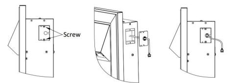
5.4b Carefully mark out the fixing screw positions as below, fit two ST4\*12 screws leaving approximately 4mm between the wall/panel and the screw head.
