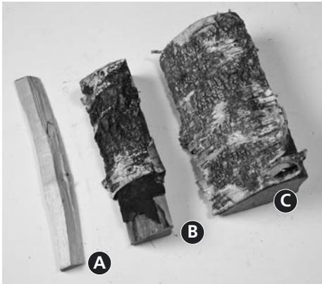
*The recommended maximum fuel load: Photo shows a typical loosely stacked fuel load of approximately 1.75kg of fully seasoned wood logs approx 350mm (14") long by 75 – 100mm thick*
