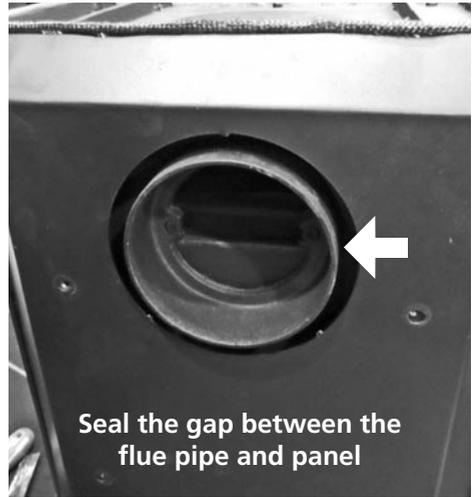
*To maintain good convection it is essential that the gap between the flue pipe and the cut-out on the heat shield is sealed by either using fire rope and / or fire cement.*
