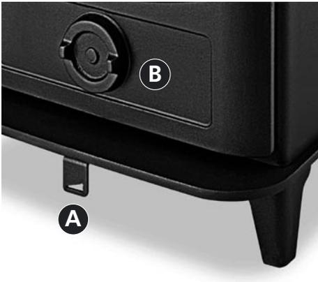
Use the tool provided to adjust the Secondary air control A – moving it to the left hand side will reduce the air supply and ‘slow’ the fire down. B is Primary air – move clockwise to close
