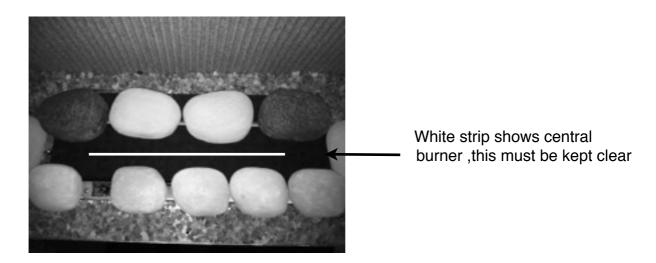
The four pebbles marked L sit at the rear of the base pad and on to the fibre strip as left above The final 2 pebbles sit at the side as above .
