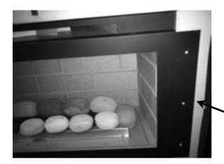
THE GLASS IS HELD IN PLACE BY THE FIXING FRAME AND CAN BE REMOVED BY REMOVING THE SCREWS ON THE LEFT AND RIGHT SIDES
