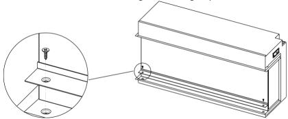
Unscrew the four ST4\*8 screws on both sides of the appliance, and remove the top brackets as shown below, ensuring the glass panel is supported all the time.
