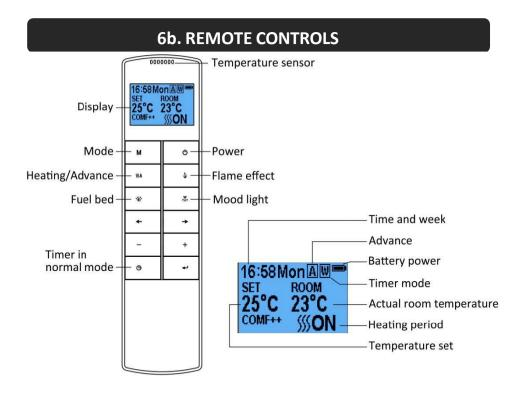
NOTE: This is a thermostatic remote control. The remote should be in the same room as the fireplace and placed on a flat surface. It must be placed away from the fire so the hot air will not blow on it and affect the thermostatic reading.
