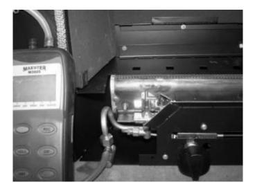
Check that the inlet gas pressure is at 20 mbar
