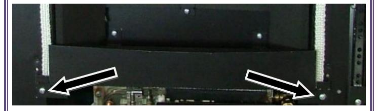
Now you can remove the tray for a manual tray remove the two screws
