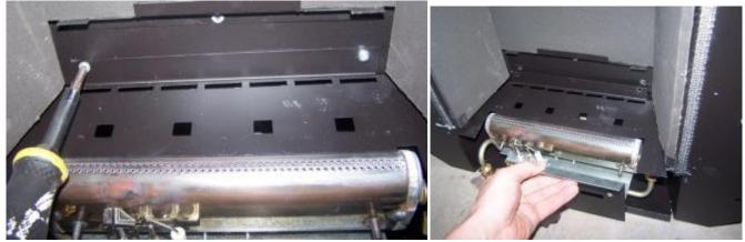
The tray is now free and may be lifted away from the box, lift free of the retaining clips on each side of the burner tray.
