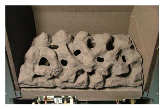
Once the fuel bed is in position you can the refit the glass support base bracket and gentle place the glass into position, then fit the top retaining bracket with the three screws **DO NOT** over tighten.
