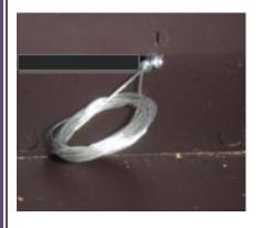
Surplus tension cable **MUST NOT** be cut off as this will prevent proper installation after servicing simply coil up the surplus cable as shown and tuck the coils out of the way.
