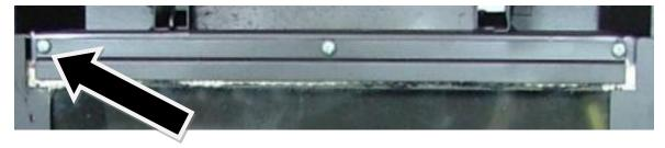
Now remove the two screws holding the base glass panel support.
