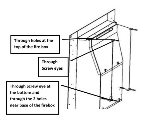
Push the appliance back into the fireplace, centralise and pull the loose cables through the holes into the firebox, thread the cable tensioners onto the cable as shown, with the nuts screwed down close to the tensioner head. Slide the screwed nipple through the box and pull cable taut and tighten pinch screw on to the cable.
