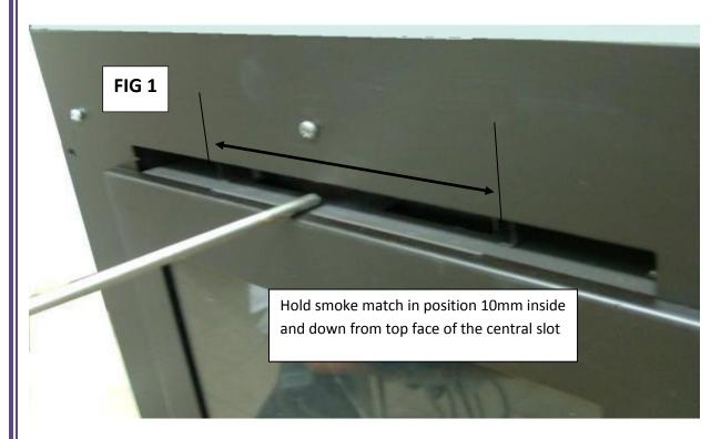
When the test has been completed satisfactorily, repeat with any extractor fans in the premises running on the highest setting, and any communicating doors open.
