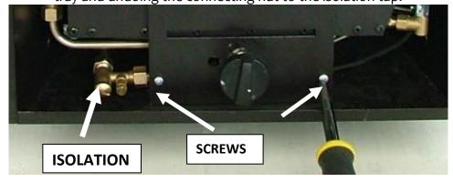
Now, remove the 2 screws on the top of the burner tray.
