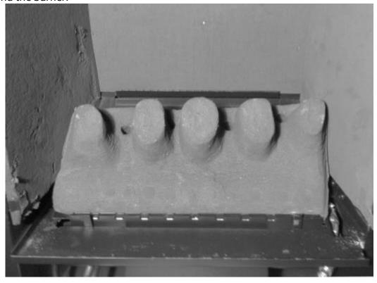
Place the rear matrix behind the middle matrix and again ensure it is sitting flat on the base plate of the burner.
