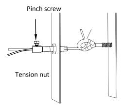
Adjust tensioner using a suitable spanner to pull the cable tight into position, to allow an even seal around the edge of the fire, visually inspect the seal and reseat if necessary.
