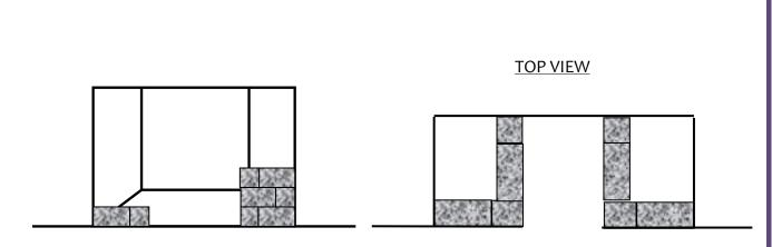
Any type of fire surround used with this appliance must be adequately sealed to the wall and floor; a combustible shelf may be fixed to the wall above the fire, providing that it complies with the dimensions given below.
